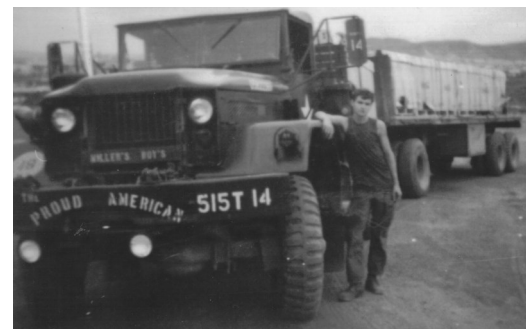
Specialist 4 Robert Newell, of the 515th Transportation Company with his truck, "The Proud American". His five-ton truck is augmented by a fifth wheel dolly, to carry 20 more tons of supplies.
